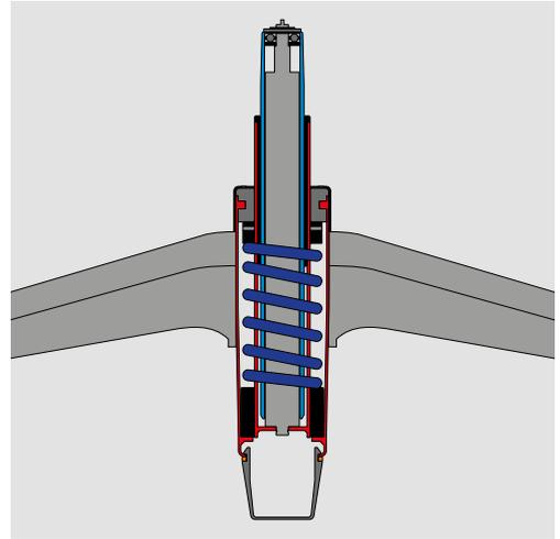
**Soft as a feather.** Thanks to the patented Sedo Lift mechanism, the seat height adjusts easily and continuously. At the same time, soft, pleasant, back-friendly cushioning is guaranteed regardless of the chosen seat height. However, the Sedo Lift mechanism is not only extremely comfortable, but also non-wearing and thus highly durable.
